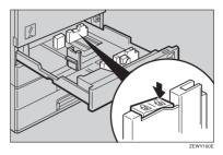
While pressing the release lever, adjust the side guides.
